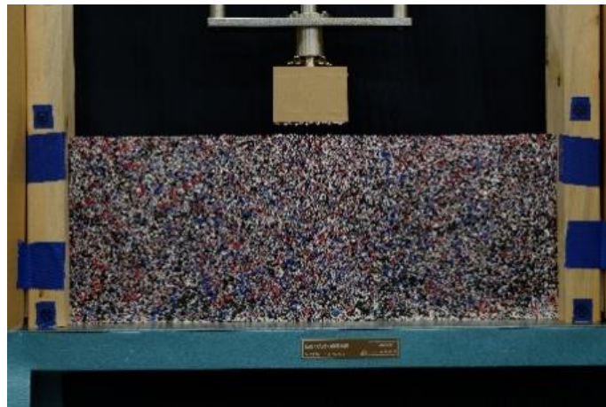
Figure 6 : Arrangement of shallow foundation loading test equipment
