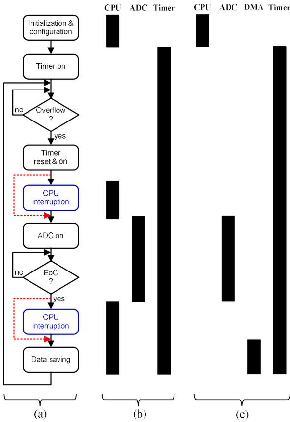
Fig. 2. (a) Flowchart of the measurement process; differences between ISR and PTP techniques are highlighted in blue solid line and red dashed line, respectively. Time intervals in which the embedded resources are activated when applying the (b) ISR, and (c) PTP techniques.
