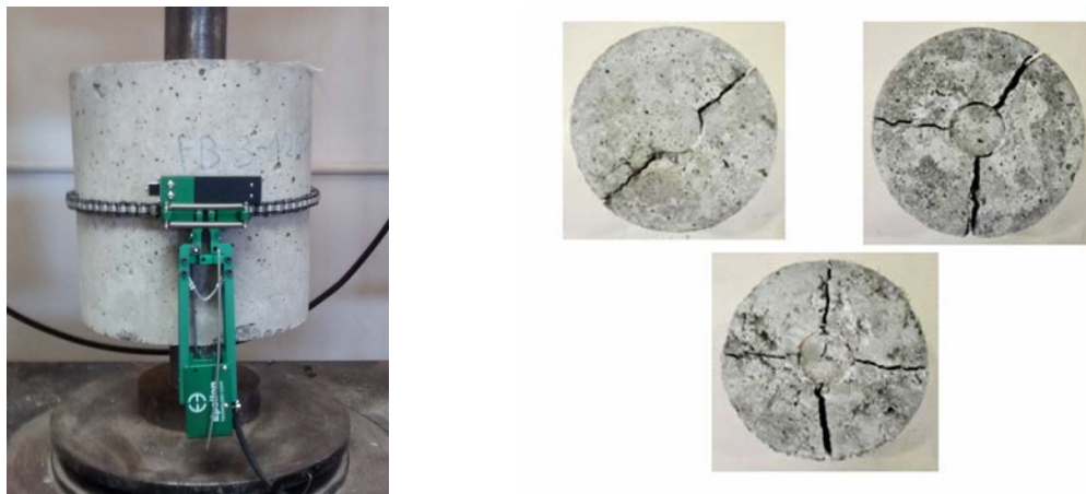
Figure 4. (a) BCN test setup; (b) Typical final state of specimens subjected to double punching tests.
