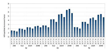
Fig. 10 MFlops per Watt improvement (more is better) for Streamcluster with different combinations of core count, reg. size, and frequencies (scalar, vector and LLC).
