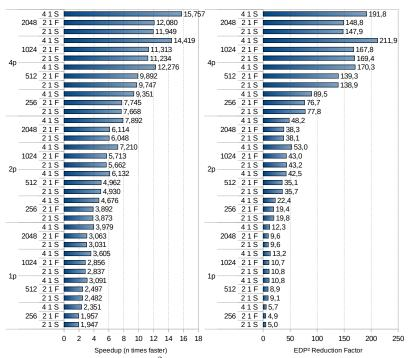
Fig. 11 Speedup (left) and  $EDP^2$  improvement (right) for Swaptions (more is better) normalized to 1 core with 128-bit registers running at 1Ghz with slow LLC. Y axis shows different combinations of core count, reg. size, and frequencies (scalar, vector and LLC).
