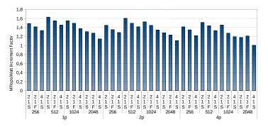
Fig. 14 MFlops per Watt improvement (more is better) for Vreduction with different combinations of core count, reg. size, and frequencies (scalar, vector and LLC).
