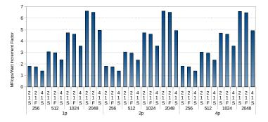
Fig. 12 MFlops per Watt improvement (more is better) for Swaptions with different combinations of core count, reg. size, and frequencies (scalar, vector and LLC).
