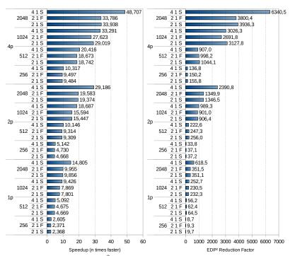
Fig. 3 Speedup (left) and  $EDP^2$  improvement (right) for Blackscholes (more is better) normalized to 1 core with 128-bit registers running at 1Ghz with slow LLC. Y axis shows different combinations of core count, reg. size, and frequencies (scalar, vector and LLC).
