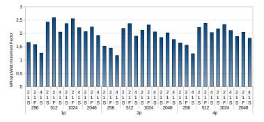
Fig. 7 MFlops per Watt improvement (more is better) for Matmul with different combinations of core count, reg. size, and frequencies (scalar, vector and LLC).
