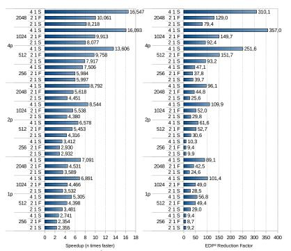
**Fig. 6** Speedup (left) and  $EDP^2$  improvement (right) for Matmul (more is better) normalized to 1 core with 128-bit registers running at 1Ghz with slow LLC. Y axis shows different combinations of core count, reg. size, and frequencies (scalar, vector and LLC).
