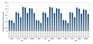
Fig. 4 MFlops per Watt improvement (more is better) for Blackscholes with different combinations of core count, reg. size, and frequencies (scalar, vector and LLC).
