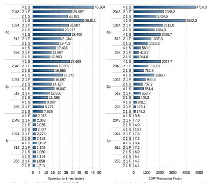
Fig. 9 Speedup (left) and  $EDP^2$  improvement (right) for Streamcluster (more is better) normalized to 1 core with 128-bit registers running at 1Ghz with slow LLC. Y axis shows different combinations of core count, reg. size, and frequencies (scalar, vector and LLC).
