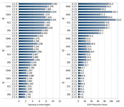
Fig. 13 Speedup (left) and  $EDP^2$  improvement (right) for Vreduction (more is better) normalized to 1 core with 128-bit registers running at 1Ghz with slow LLC. Y axis shows different combinations of core count, reg. size, and frequencies (scalar, vector and LLC).
