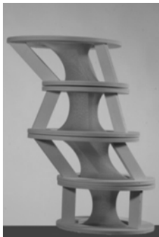
Fig. 01 Physical study model showing catenoids between shifted circular rings
