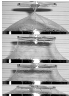
Fig. 02 Sequence of Soapfilm Models
