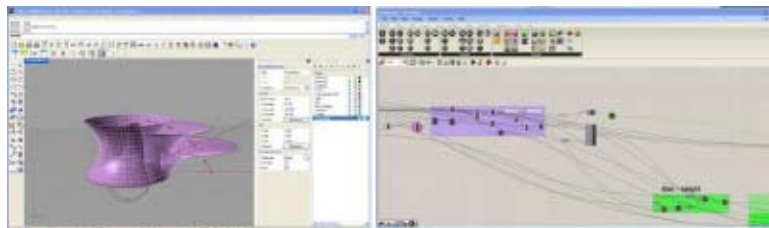
Fig. 47 Grasshopper script “Catenoids between horizontally shifted circular rings”
