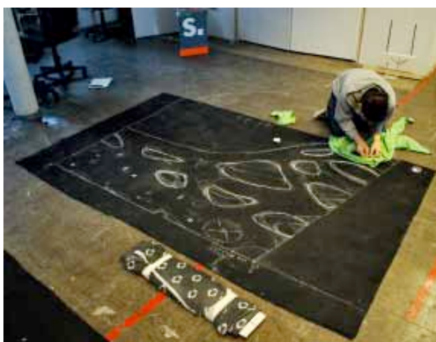
Figure 11 Layout and marking of formwork
