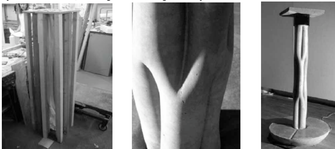
Figure 7 Undulated surface in column created by laser cut plywood ribs
