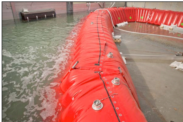
Figure 7: Laboratory test of the prototype Daedler within the research project HWS-MOBILE (photo: B. Koppe)
