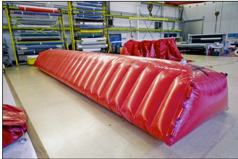
Figure 4: Tube system prototype with inner reinforcements made by the company Karsten Daedler in Trittau, Germany (photo: M.W. Jürgens)
