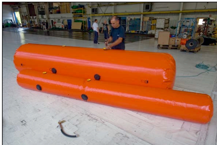
Figure 5: Tube system prototype made of two jointed cylindrical tubes made by the company Optimal in Menden, Germany (photo: M.W. Jürgens)
