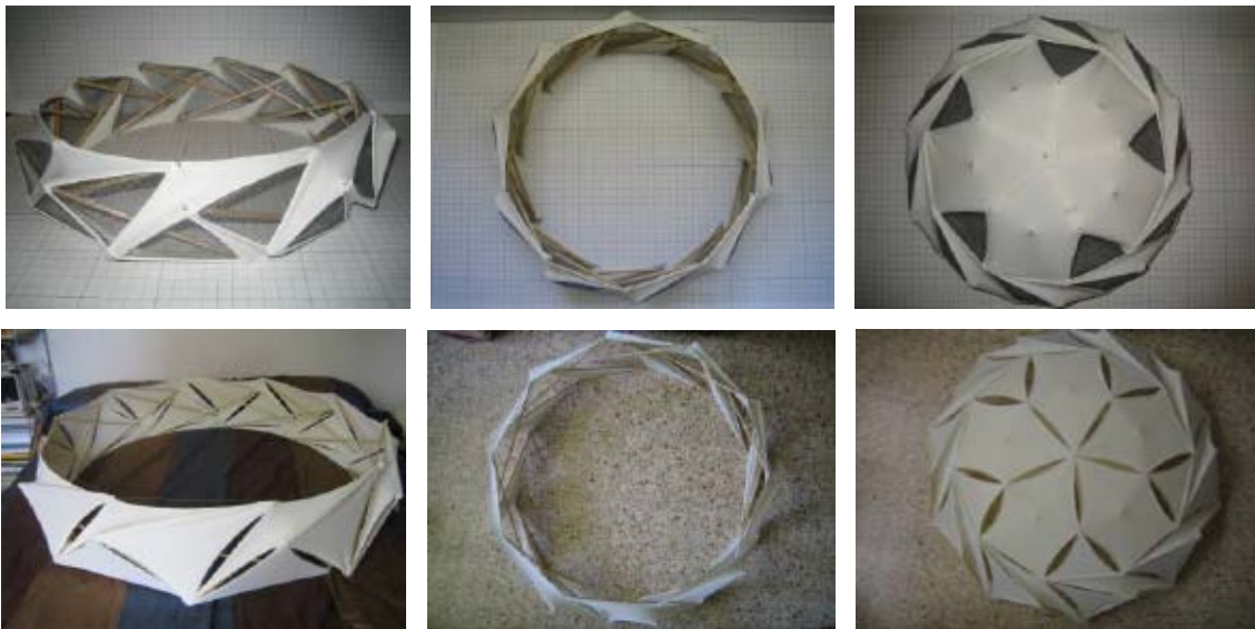
Figure 1: Tensegrity ring diameter Ø 40 cm. (above) - Tensegrity ring diameter Ø 100 cm. (below) - Models scale 1:100
