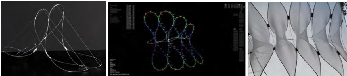
Fig. 6: Spring-based computational modelling of internal cell logic. Cell assembly in final structure.
