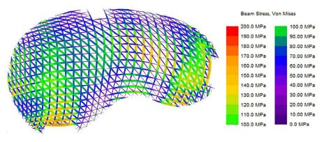
Figure 6: Stress resulting from forming in the Soliday's gridshell
