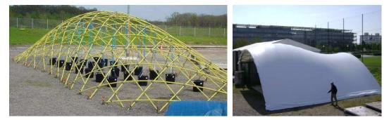
Figure 5: a. First experimental gridshell under testing. b. Second experimental gridshell used as a shelter for a wind tunnel.
