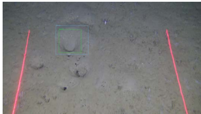
Figure 2.2.7: Ground-truth vs. Model Detection- Cadiz.
