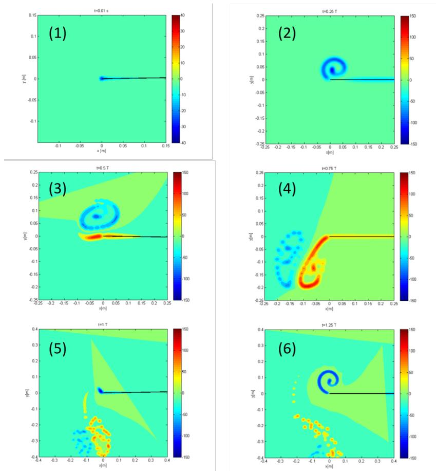
Figure 4: Snapshots of the vorticity field at time  $t=0.01T$  (1),  $t=0.25T$  (2),  $t=0.50T$  (3),  $t=0.75T$  (4),  $t=1.00T$  (5),  $t=1.25T$  (6) obtained from a forced-oscillation simulation of the 1d-membrane example ( $a_0/L=0.005$ ).  $T$  is the entire oscillation period. The visible frame represents a small area in the vicinity of the left edge (see Figure 5). The membrane and the time series of its prescribed motion are displayed in Fig. 5.
