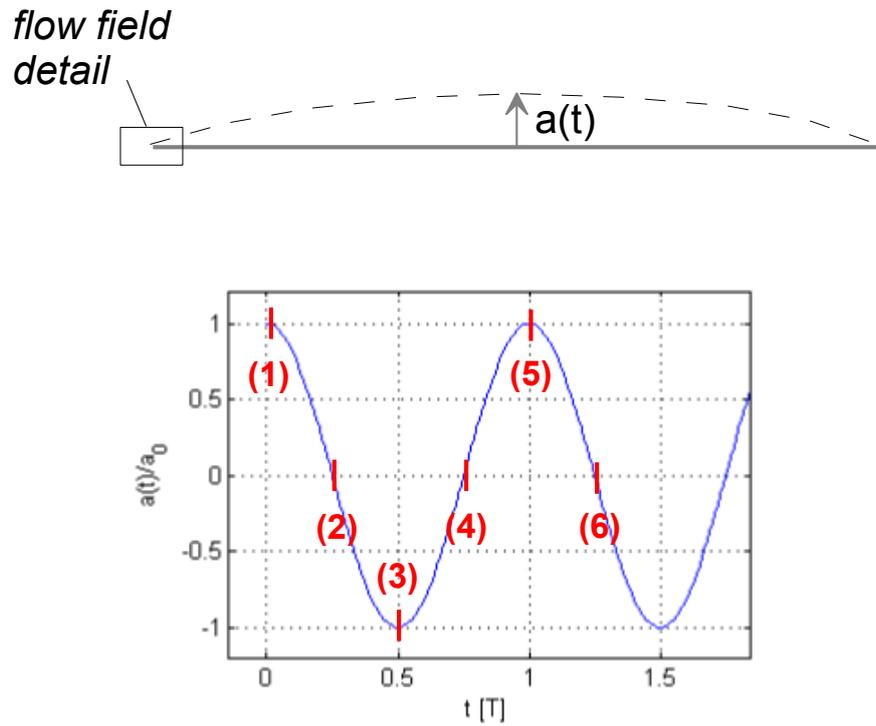
Figure 5: Sketch of the test case (1d-membrane with sinusoidal eigenmode) with indication of the detail frame shown in Figure 4 (upper image) and display of the membrane motion time series including indication of the snapshot times of images 1 to 6 in Figure 4 (lower image).
