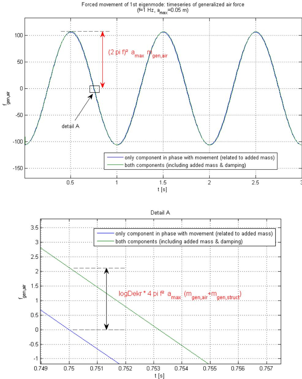
Figure 3 : Time series of the reaction force obtained from a forced-oscillation simulation of the 1d-membrane example and geometrical interpretation of the target parameters  $m_{gen,air}$  and  $\delta_{air}$ . As shown in the detail (lower image), the phase of the overall generalized force (green line) is somewhat shifted from the membrane motion.
