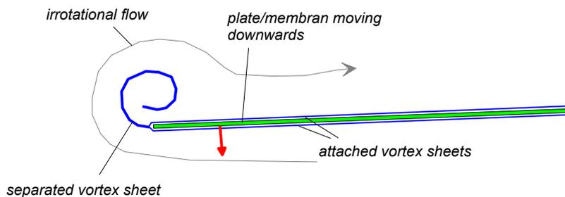
Figure 2: Formation of the spiral vortex immediately after the onset of downward motion of the object (symbolized by the red arrow)
