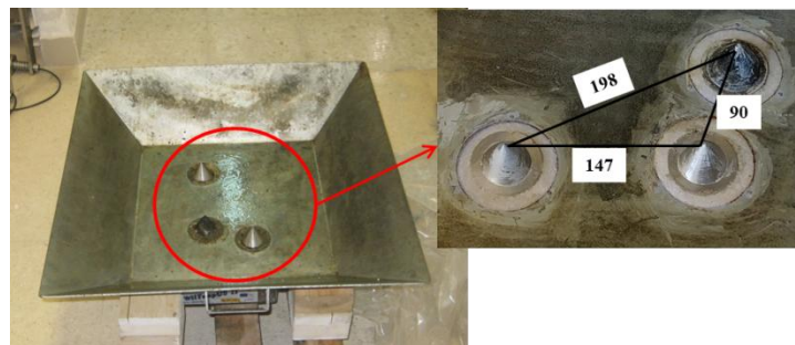
Figure 4. Position of the transducers in the trough.
