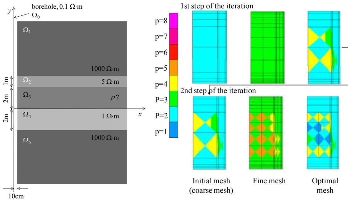
**Figure 2:** a) The 2D geometry of 3D DC borehole resistivity measurements problem. The rock formation is composed of five different layers of various resistivities, b) Automatic  $hp$ -adaptive solver – a solution example.
