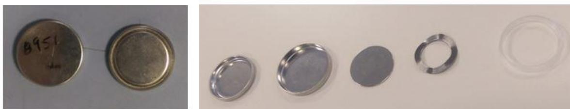
Figure 2 Photos of the cells manufactured by IREC (left) and their individual parts (right).
