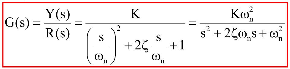
with K: system gain (corresponds to final value for a unit step function)
