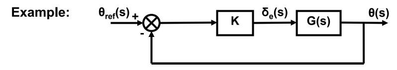
Compute the error in steady state for a unit step function
