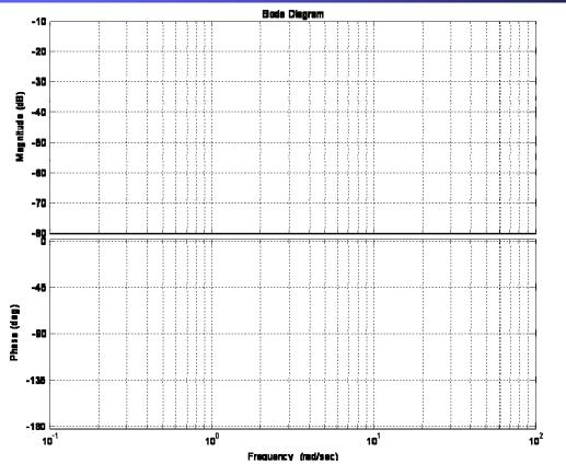
Semi-logarithmic axes: with lineal scale for the magnitude or the phase, and logarithmic for the frequency
