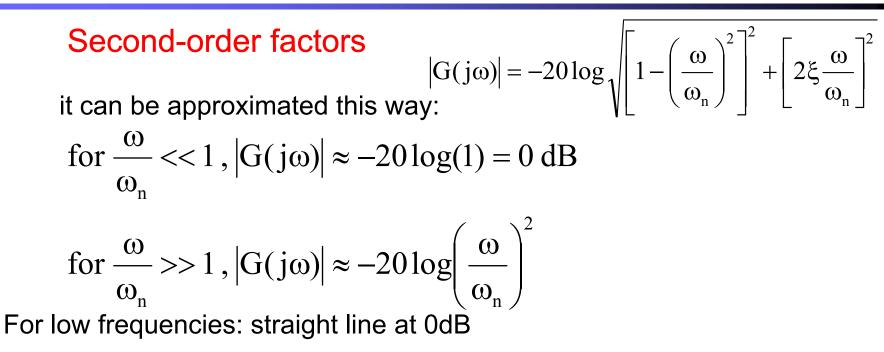
For high frequencies: straight line with a -40 dB per decade slope.
