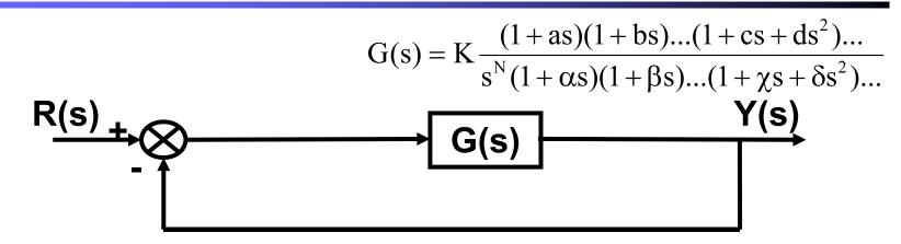
1. Position error: error for a step function entry: r(t)=u(t)
