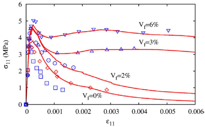
Figure 3: Uniaxial tensile test data for FRC with  $V_f = 2, 3$  and 6% of PVA fibers [12] and their simulation by the model M7f. The data for plain concrete under uniaxial tension is also shown for comparison.
