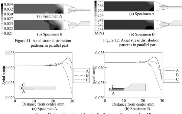
Figure 13: Transitions in axial strain distribution in Specimens A and B
