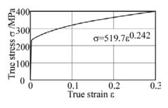
Figure 6: Ture stress-strain diagram simulation used
