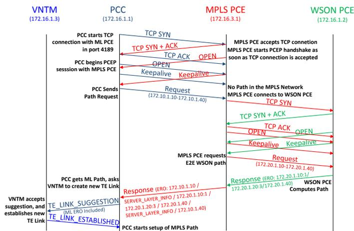
Fig. 2. Multi-PCE/VNTM signaling for coordinated multi-layer path computation. Note that in this example, the IP addresses of the PCC and the source node within the path computation request differ. As mentioned above, this is because the PCC could be an NMS. In the next section, we will examine this case in further detail.
