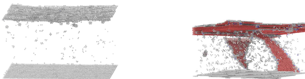
Figure 2: The structure of the samples after irradiation of the \{100\} (a) and \{111\} (b) surfaces.
