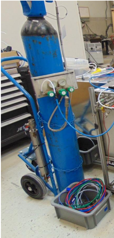
Fig. 14: Bombona de N 2 (200 bar)
