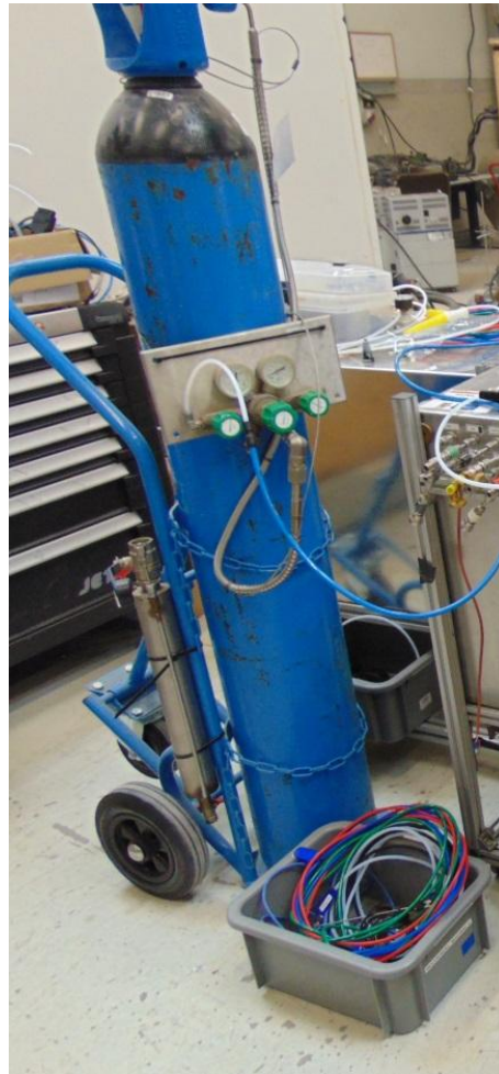
Fig. 26: Bombona de N 2 (200 bar)
