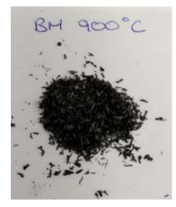
Figure 37. Char obtained with Biomass at 900°C
