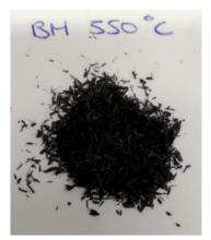
Figure 35. Char obtained with Biomass at 550°C
