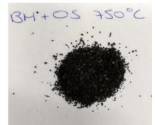
Figure 42. Char obtained with Biomass and Oil Shale at 750°C
