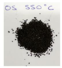
Figure 38. Char obtained with Oil Shale at 550°C
