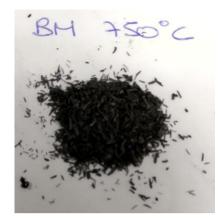
Figure 36. Char obtained with Biomass at 750°C
