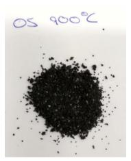
Figure 40. Char obtained with Oil Shale at 900°C
