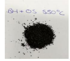
Figure 41. Char obtained with Biomass and Oil Shale at 550°C
