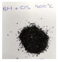
Figure 43. Char obtained with Biomass and Oil Shale at 900°C
