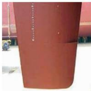
Figure 38: Twisted Leading Hedge Rudder on the CMA-CGM Containership CHRISTOPHE COLOMB. Figure by "eagle.org".
