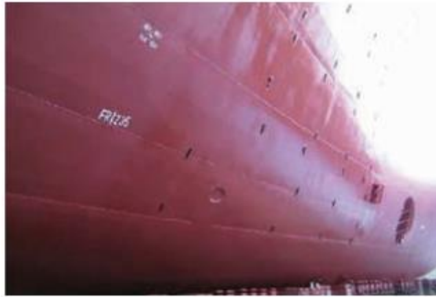
Figure 50: OLIVIA MAERSK Showing Wing Air Induction Pipe Micro-bubble Units Staggered Over its Side. Figure by "maersk.com".
