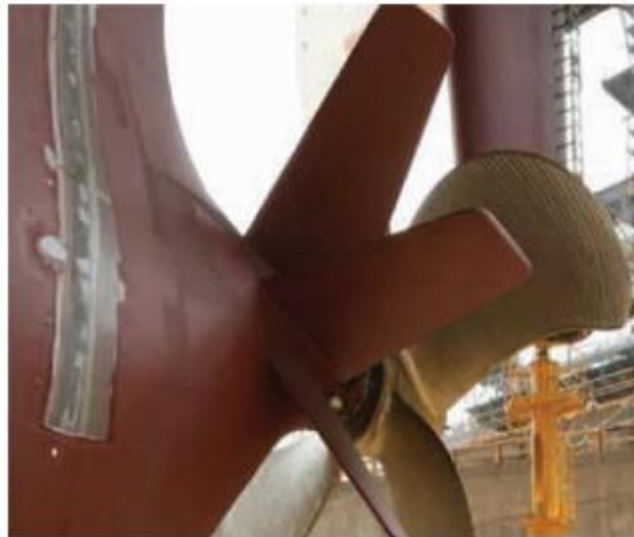
Figure 36: Stators on CMA-CGM Containership CHRISTOPHE COLOMB. Figure by "eagle.org".
