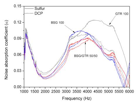
Figure 8. Sound absorption coefficient as a function of frequency for NR/BSG/GTR biocomposites.
