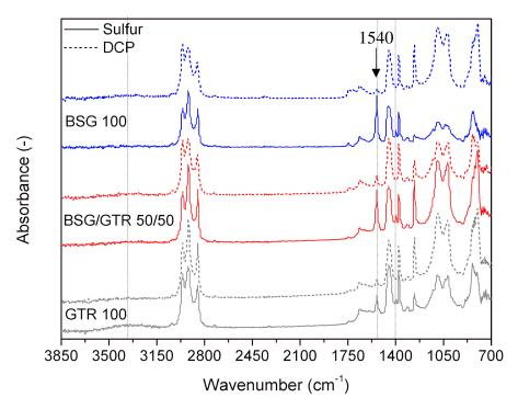
Figure 4. FTIR spectra for NR/BSG/GTR biocomposites.
