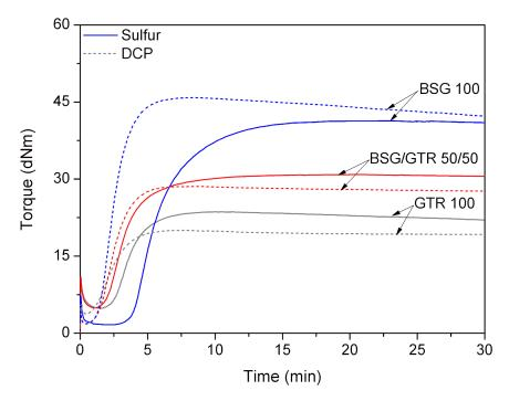
Figure 3. Curing curves for highly-filled NR/BSG/GTR composites.
