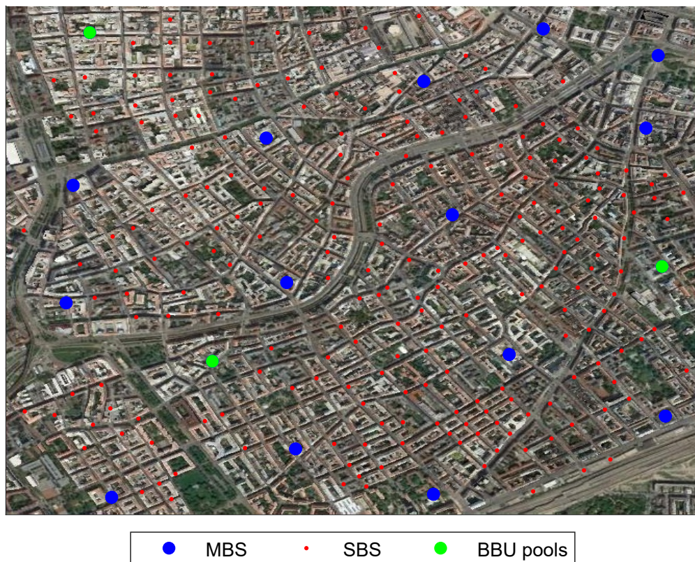
Figure 4.3 C-RAN deployment over Vienna city downtown. Green points represent BBU pools location while blue and red marks are MBSs and SBSs (RRHs), respectively.
