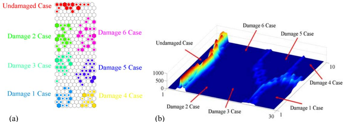
Figure 5. Analysis with fused PCA, SPE and SOM: (a) Cluster Map and (b) U-Matrix Surface.
