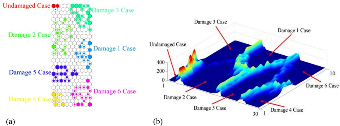
Figure 6. Analysis with fused h-NLPCA, SPE and SOM: (a) Cluster Map and (b) U-Matrix Surface.
