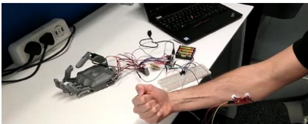
Figure 10: EMG control test of the hand using a pushbutton to switch the type of grasp [13].
