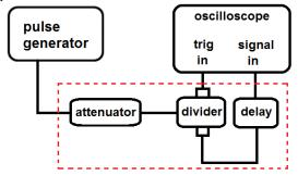
Fig. 5. Typical measurement setup for the calibration of the pulse generators using equivalent-time sampling oscilloscope.
