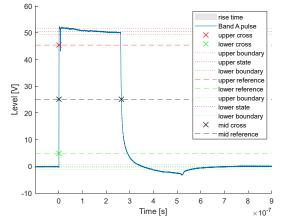
Fig. 2. Calibration pulse generated by the IGUU 2916 for CISPR band A
