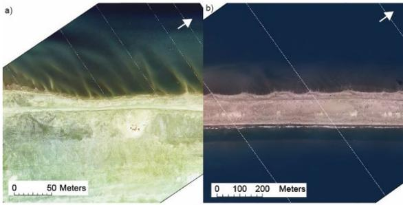
FIGURE 2. (a) Transverse bar system in 2012; (b) large scale undulations in 2013. Source: ICGC
