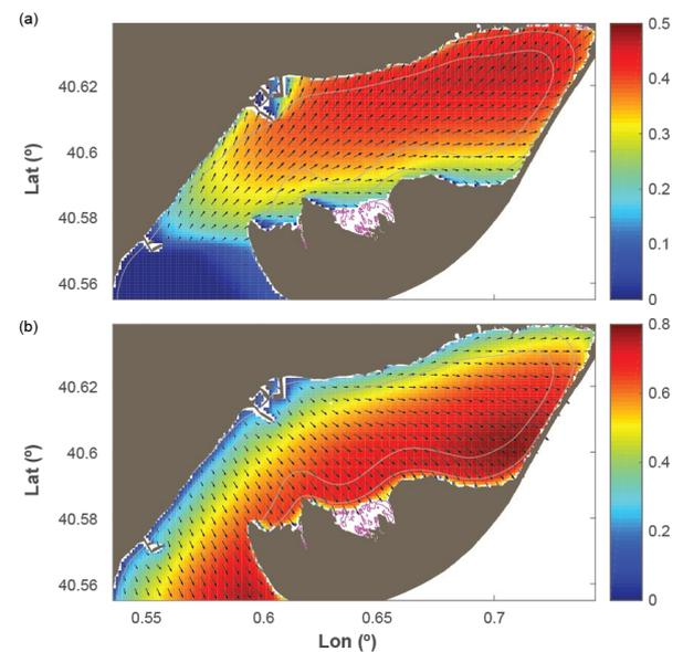
FIGURE 1. Spatial distribution of the significant wave height and wave direction of propagation obtained with SWAN model. (a) SW events with 9 m/s of wind speed (b) NW events with 15 m/s of wind speed.
