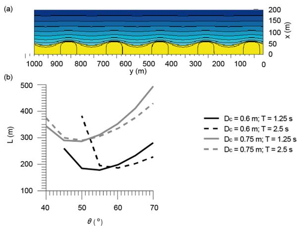
FIGURE 6. Results obtained from 1D morfo model. (a) plain view of large-scale undulations of 200 m wavelength with bathymetric lines every 0.1m (amplitude value in the model = 10m), (b) dominant wavelength (black:  $D_c = 0.6$ , gray:  $D_c = 0.75$ ; continuous:  $T = 1.25$ ; dashed  $T = 2.5$ )
