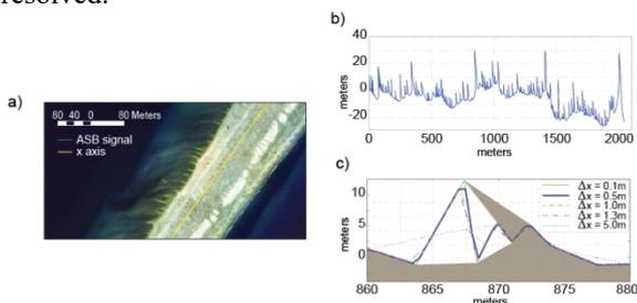
FIGURE 3. Methodology used to analyze the evolution of the shoreline. (a) In yellow: signal obtained from the manual profiling; (b) Signal obtained after rotating the original data; (c) Interpolation of equi-spaced points using different  $\Delta x$ .
