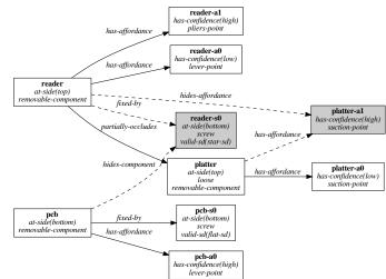
Fig. 4. Device with unseen components and relations (total occlusions). Namely, *pcb* is hiding some screws that are fixing the *reader* component at the opposite side of the hard drive. This corresponds to a real-life model.
