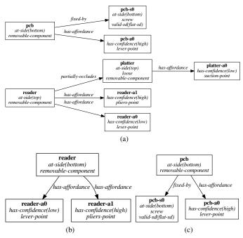
Fig. 3. (a) Device with partial occlusions. The only components eligible for retrieval are *reader* and *pcb*. (b) and (c) show the simplified state that results from focusing on each of these, respectively.
