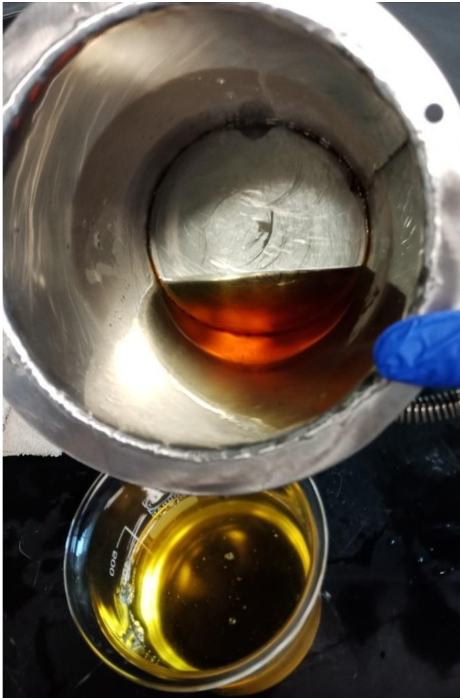
Figure 6. Purified biodiesel (gold coloured liquid) and glycerol (dark coloured liquid) after SAC process
