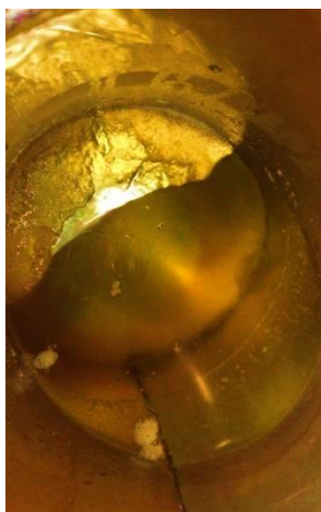
Figure 5. Solid glycerol and liquid biodiesel in the cylindrical vessel
