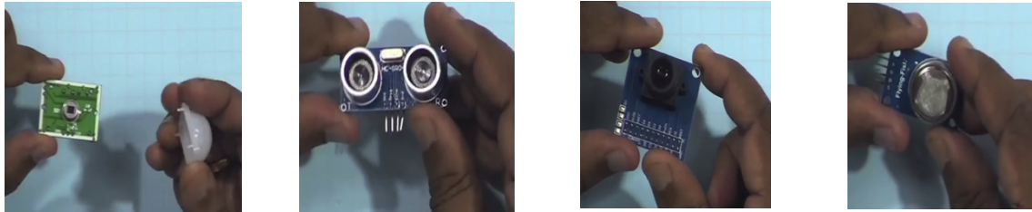
Figure 9. Examples of different sensors: obstacle detection, ultrasonic, camera sensor and temperature sensor
