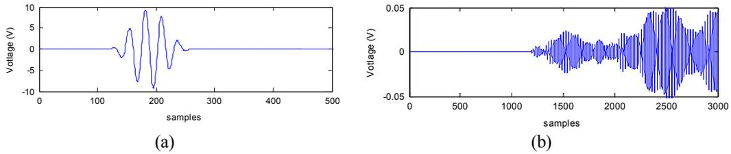
*Figure 2. Generated and received waves, a) tone burst actuating signal b) received signal.*
