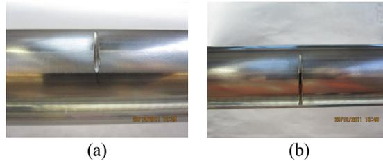
*Figure 3. (a) and (b) two example of saw cuts in pipe structure with different severities.*
