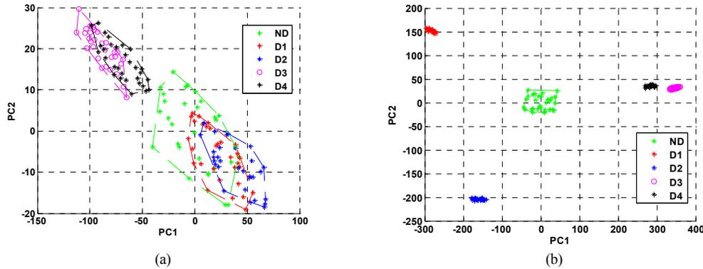
Figure 5. Route 1-6 from actuator 1 to sensor 6 a) PCA cannot separate the pattern of damages from the healthy one b) complete separation is satisfied.
