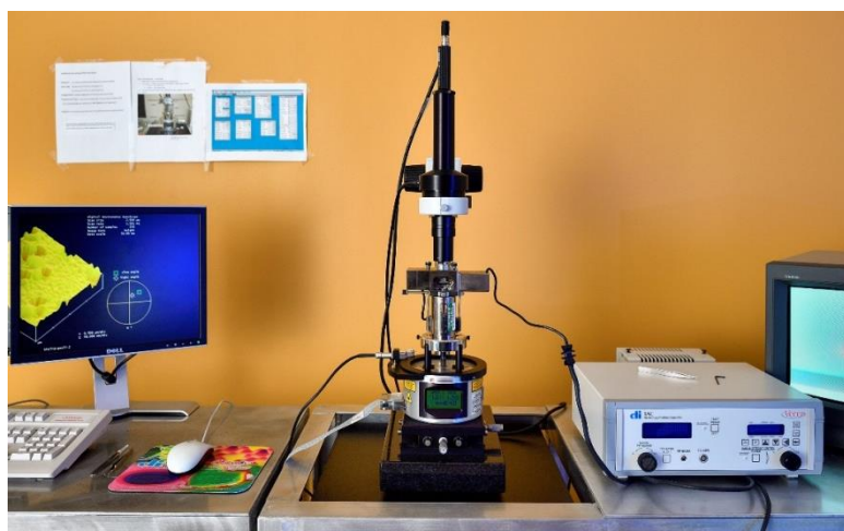
Figura 26. Microscopi de sonda de rastreig TM-AFM NanoScope IIIa Multimode de Digital Instruments.
