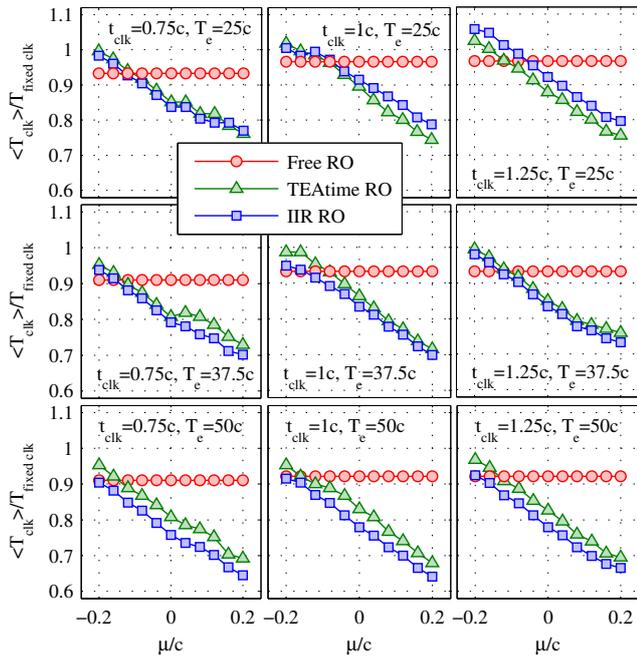
Fig. 8. Relative adaptive period for different CDN delay and variation period values when there is a static mismatch  $\mu$  between the RO and the TDC. On almost any situation the IIR RO is the architecture that ensures the greatest safety margin reduction. Only for high frequency HeDV (upper row) TEAtime RO or free RO surpass the IIR RO when  $\mu/c < -0.1$ .
