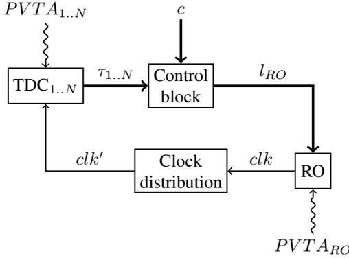
Fig. 2. Closed loop controlled ring oscillator architecture. The main signals are labelled: the set-point  $c$  which is the only input of the clock generation system, the ring oscillator length  $l_{RO}$ , the generated clock  $clk$ , the distributed clock  $clk'$  and the  $i$ -th TDC lecture  $\tau_i$ . Also we point out that the clock generator, the RO, and the sensors, the TDCs, could suffer different variations.
