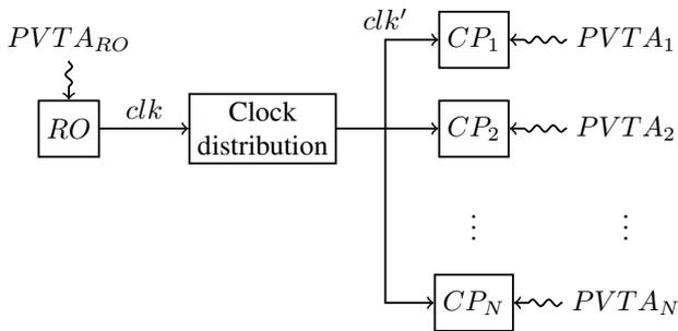
Fig. 1. Free running ring oscillator (RO) used as a self-adaptive clock generator. The main elements that undermine the performance of RO as a self-adaptive clock generator are depicted: the mismatch between the variations suffered by the RO and the circuit critical paths (CP); and the clock distribution network which introduces a delay between the generated and the delivered clock signal to the CPs.
