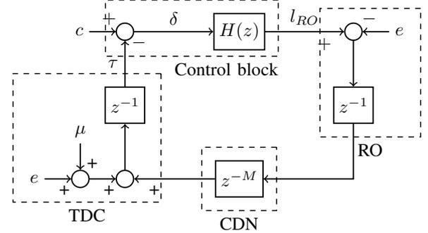
Fig. 3. Discrete system view of the closed loop controlled ring oscillator. The main blocks of the architecture are labelled. The system inputs are labelled: the set-point  $c$ , homogeneous variation  $e$  and heterogeneous variation  $\mu$ . As well as important signals: RO length  $l_{RO}$  and adaptation error  $\delta$ . The CDN number of samples  $M$  delay depends on the input value to the CDN block and the CDN delay in number of stages:  $M = \lceil t_{clk}/T_{clk} \rceil$ .
