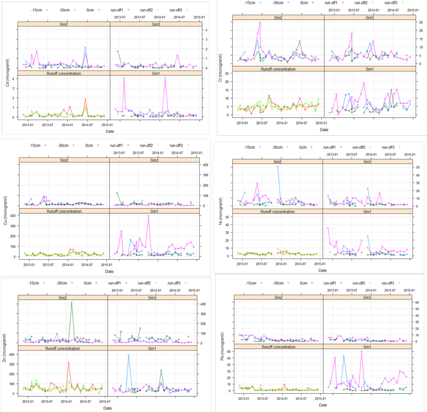
Figure 2. Raw data of the dissolved soil solution concentrations of the three different embankment soils and the runoff concentrations during the measurement period
