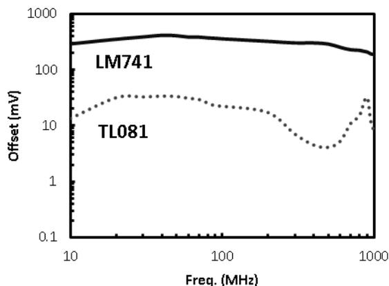
**Fig. 2.** Operational amplifier offset voltage when a RFI interference of 0 dBm is injected at the inverter input at room temperature.
