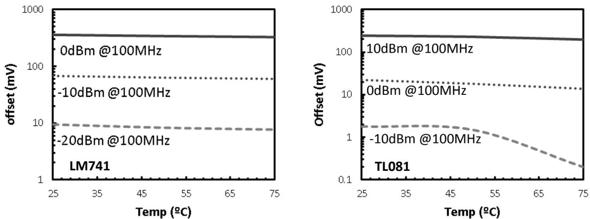
**Fig. 4.** Operational amplifier offset voltage temperature dependence. The results are show for three different RFI power injection levels.
