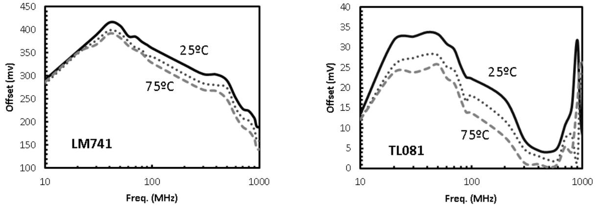
**Fig. 3.** Operational amplifier offset voltage when a RFI interference of 0dBm is injected at the inverter input ( $f=100$  MHz). The results are shown for three temperatures: 25°C, 50°C and 75°C.
