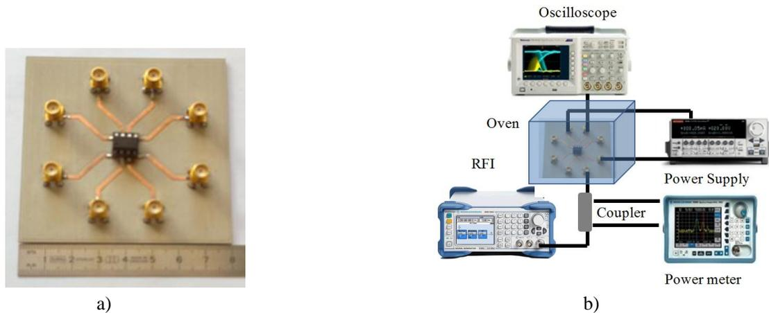
**Fig. 1.** a) PCB specifically designed for this experiment. b) Experimental setup
