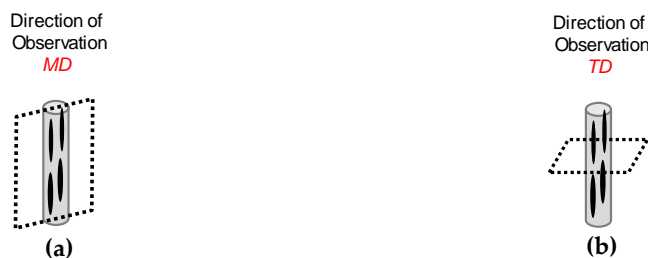
Figure 4. Scheme of the observation directions for the morphology analysis: (a) melt flow direction (MD); (b) transversal to melt flow direction (TD).
