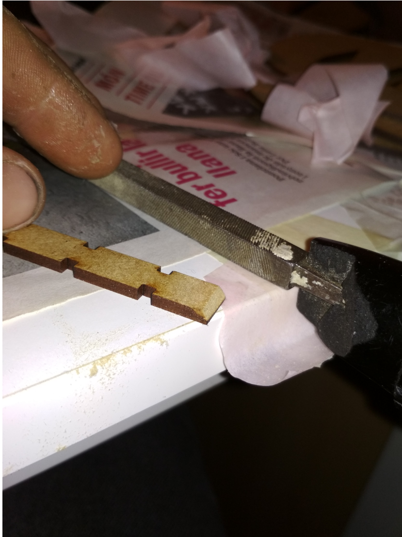
Figure 25: Realization of a chamfer to adjust the vertical stabiliser
