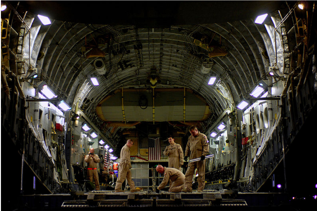
Figure 4: Image of the C-17's formers [2]
