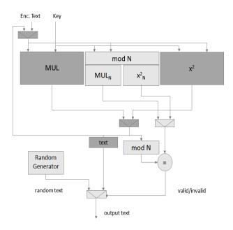
Figure 1. Block Diagram of RSA + Protection Circuit
