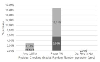
Figure 4. Area and power increase for RSA + Resiude Checking mechanism
