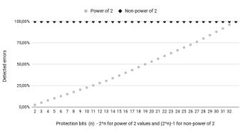
Figure 3. Detection capabilities as a function of the modulo value
