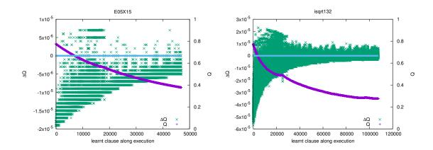
Figure 2: Impact of adding learned clauses on modularity, in instances E05X15 (left) and  $isqrt1_32$  (right). Each point (x, y), with y measured in the left Y axis, represents a clause learned at instant x and increasing Q on y. We also represent the evolution of the modularity Q (using the right Y axis).
