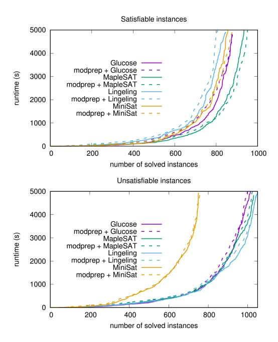
Figure 3: Cactus plot representing the results of the solvers Glucose, MapleSAT, Lingeling and MiniSat with and without using the modularity-based preprocessor *mod-prep*, on the aggregated set composed of all application instances from the SAT Competitions from 2010 to 2017, distinguishing between satisfiable (top) and unsatisfiable (bottom) instances.
