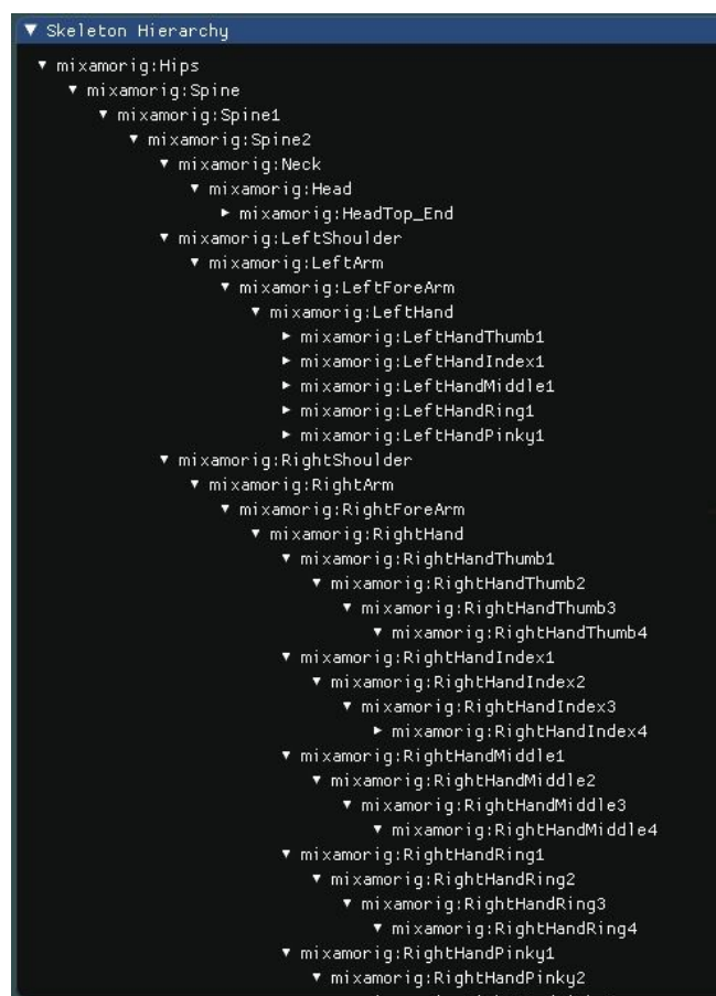
F5.21 Skeleton hierarchy - Shows the relation between the different joints in the skeleton
