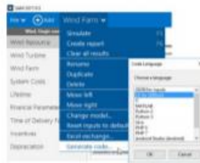
Figure 2. The Generate Code command on the Case menu exports ready-to-run code from the desktop application to use with the software development kit.
