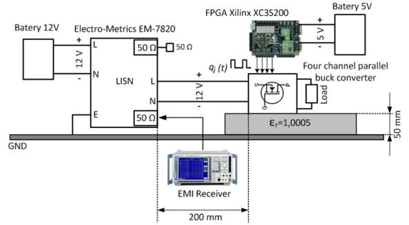
Figure 5: EMI measurement set-up
