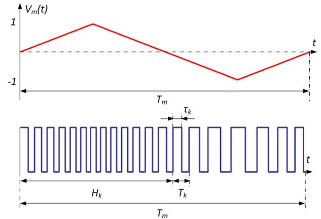
Figure 1: Spread Spectrum Modulation with periodic modulation profile
