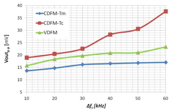
Figure 9: Output voltage ripple vs  $\Delta f_c$
