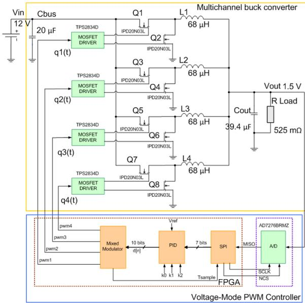
Figure 4: Block diagram of the experimental plant.
