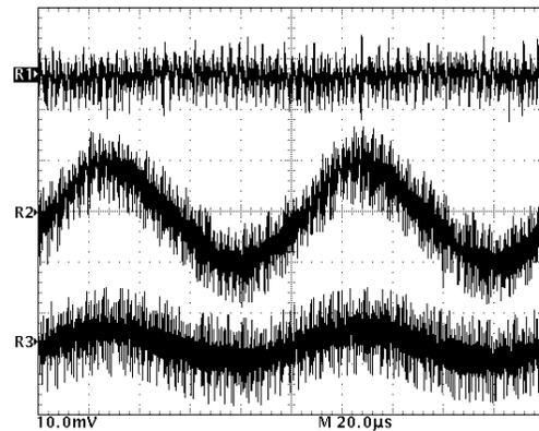
Figure 8: Output voltage ripple comparison: CDFM-Tm, CDFM-Tc and VDFM (R1: CDFM-Tm; R2: CDFM-Tc; R3: VDFM)
