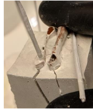
Figure 32. Broken Wire in sample 0.8_4.
