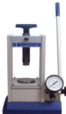
Figure 21: Hydraulic press ( Specac ) employed for the powder compacting.
