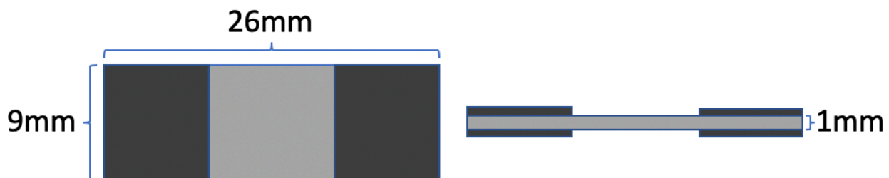
Fig. 1. Illustrations of the employed sample. The geometry of the sample is 26x9x, with graphite glue applied on the two extremes.
