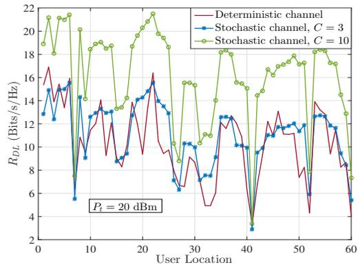
Fig. 6: DL SE vs users locations based on stochastic channels (average over 1000 realizations) and deterministic ray based channels at  $N_t = 128$ ,  $N_r = 32$ ,  $C = \{3, 10\}$ ,  $P_t = 20\text{dBm}$  and  $\sigma^2 = -84\text{dBm}$ .
