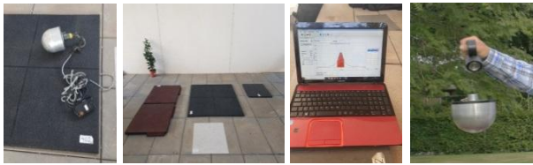
Figure 10. HIC meter Wireless Impact Test-1177-2018- By author
