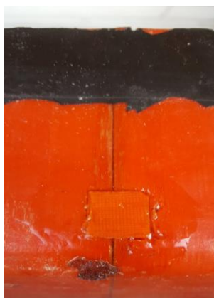
Figura 6: Tancament tanc reparat
