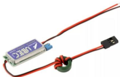
Figura 31: Hobbywing 3A UBEC 5V 6V 0
